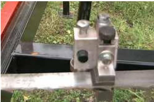
4. Our blade guides constrain the blade on both the top and the bottom. Most mfgs just push the blade from one side.
